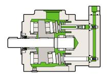
Checkball pumps are single fluid pumps with bearing lubrication provided by the pumped fluid. This eliminates the potential for fluid cross contamination, possible in other pump designs with isolated bearing lubrication. This design also eliminates the need for a separate lubrication circuit or regular maintenance of a lubricating oil.
